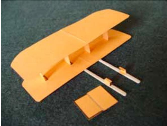
*After the wing assembly is dry, glue the elevator in place carefully. Two 5/8" long blocks of toothpick from the wider, heavier end of a toothpick should provide enough balance weight. Consult "Final Tuning For Wright Biplanes" on page 10.*
