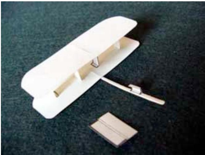
*A 7/8" block from the large end of a toothpick for weight glued to the top of your toothpick airframe should provide balance. Place it as far forward as possible. Prepare your glider to fly using the "tuning" instructions on the next page.*
