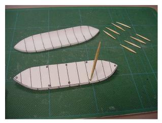
9. Set the eight short spars into the top surface of the lower elevator and add a bit of glue to each at the base as shown.
