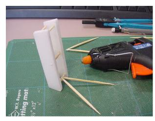
21. Stick the upper brace ends into the rear edge of the upper wing as shown and add a spot of glue. (If the wing is thin, glue the brace under the wing.) Now glue the ends of the lower brace to the rear of the skid so that the rudder is vertical.
