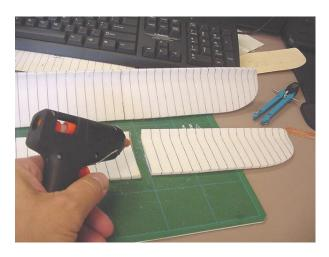
6. Use the wing template and a sharp toothpick to mark the holes for the spars on the top surface of the lower wing. Note that the front edges of the wings curve down. Dip toothpicks into glue and set them upright in the lower wing. Try not to push them all the way through the wing. Be sure they are straight and let them dry.
