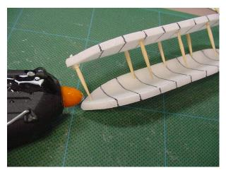
11. Print the Skids Template (page 12). Cut a 14 cm. piece of the balsa wood "A" and lay it on the template. Cut the right end at a 45 degree angle. Cut a toothpick "B" to a length of 4.5 cm., with the cut end also being at a 45 degree angle. Glue the toothpick to the balsa to form a 90 degree angle as shown. Repeat this step to make a second skid.
