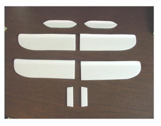
3. Use the emery board to smooth the edges. Make sure that the two halves of the upper and lower wings are flat where they will be joined, as shown at the lower right.
