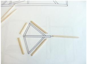
23. When dry, glue each propeller support to the lower wing 5.5 cm. from the center, in line with the back struts. Turn the Flyer over and glue to the top wing so that the support is vertical. Extra hot melt glue may be added to fill in any gap.
