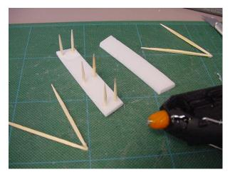
20. Glue the V-shaped braces to the rudders as shown. Once the glue is set, turn this over and glue on the other brace.
