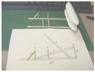
15. Now cut 2 balsa braces "C" to go from rear skid support up to elevator support. Glue them in place as shown.
