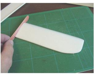
4. Using the template as a guide, take a black marker and mark the locations of the rib lines on the tops and bottoms of each wing and elevator section. Make two sets of marks, one on each edge. Connect the marks to make the rib lines. Use a permanent ultra fine black marker and a straight edge made from a manila folder (since it can be bent to conform to the rounded shape of the foam).
