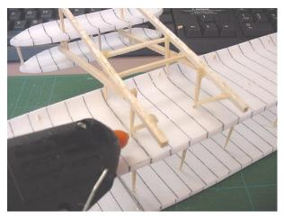
17. Cut two 10 cm. pieces of balsa "D" (see template) and sharpen one end. Glue one end under the leading edge of the upper wing between the center and next-to-center spar and then glue the other end to the bottom skid. Repeat on the other side of the skid.
