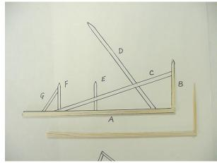
12. Turn the elevator assembly over and poke a hole through the lower elevator midway between the front and rear spars of the pairs next to the center pair of spars. Push the top of the skid assembly "A" through the hole just made, add a bit of glue, and then stick the skid into the upper elevator. Repeat with the second skid as shown.
