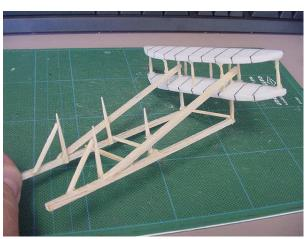
16. Turn the wing assembly over and press the skid assembly into the center of the lower wing as shown. Be sure the elevator projects out from the curved edge of the wing. Try to keep the toothpicks from going through the foam. Add some glue to each support.
