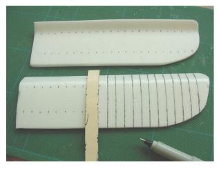
5. Place glue on the flat edge of the upper and lower wing halves and join each wing as shown.
