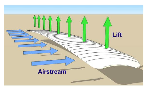
Now add the forces in play. When an airstream (represented by the blue arrows) moves over and under a wing, it generates lift (green arrows). When the wing is straight – not warped or twisted – it meets the airstream at the same angle of attack all along its length. The lift generated by the airstream is equal all along the wing. The wing is balanced around its longitudinal axis and has no tendency to roll.
