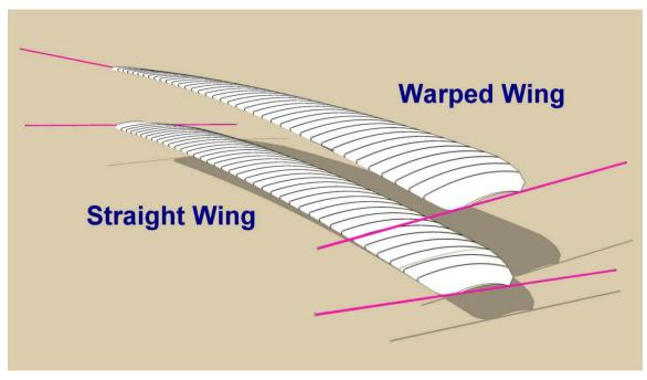
The Wright brothers' control system twisted the wings around their lateral axis. As the wings were warped, the angle of attack increased at one wing tip and decreased at the opposite wing tip.
