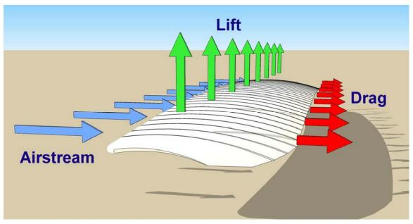
In addition to lift, the air moving over and under the wing also generates drag (red arrows), a force that impedes the travel of the wing through the air. Like lift, the drag is uniform all along the length of the straight wing. The wing is balanced around its vertical axis and has no tendency to yaw.
