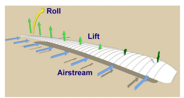
When warped, a flying wing no longer produces uniform lift along its span. In general, as the angle of attack increases, so does the amount of lift. On those sections where the airstream blows directly on the top surface, it might even produce *negative* lift (dark green arrows), pressing down on that part of the wing. With more lift on one side of the longitudinal axis that on the other, the wing wants to roll (yellow arrow).
