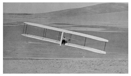
This photo is often misrepresented as Orville making a right turn. Actually, Orville is attempting to return to level flight. The right wing has dipped and Orville has moved his hips to the left, warping the wings and increasing the angle of attack on the right.
