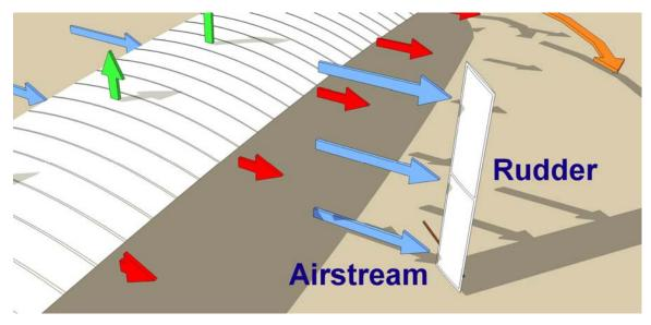
Orville reasoned that this tendency – now called *adverse yaw* – could be countered by modifying the tail and incorporating it in the control system. Convert the fixed tail to a movable rudder and turn it in the airstream toward the side of the wing that was producing the least amount of drag.
