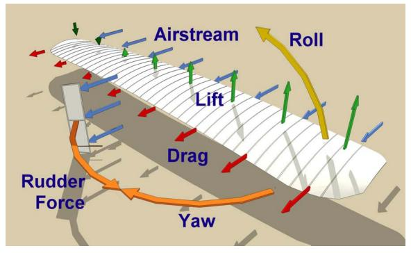
The airstream would press against the rudder surface creating a force that, when added to the unequal drag, opposed and stopped the tendency to yaw, restoring balance around the vertical axis.
