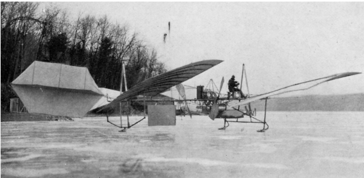
The Langley Aerodrome on 9 March 1915. The original engine has been replaced and the aircraft has been mounted on skates so it can take off from the frozen surface of Lake Keuka.
