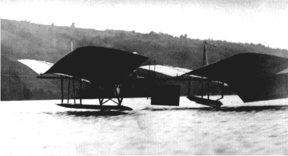
The Langley Aerodrome flies just above the surface of Lake Keuka on 2 June 1914. None of these hop-flights last more than 5 seconds or achieved an altitude of more than a few feet.
